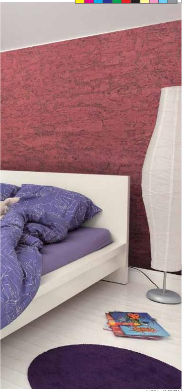
Using sheets of cork agglomerate for indoor wall coverings is a current option that allows for improved conditions of thermal and acoustic comfort in any space (image 7).
