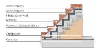
Image 5 - Use of pure expanded agglomerate in wall insulation (with air cavity)
