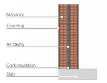
Image 6 - Use of pure expanded agglomerate in wall insulation
