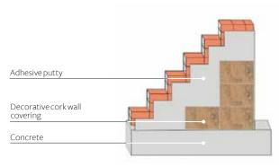
Image 7 - Use of cork for internal wall coverings
